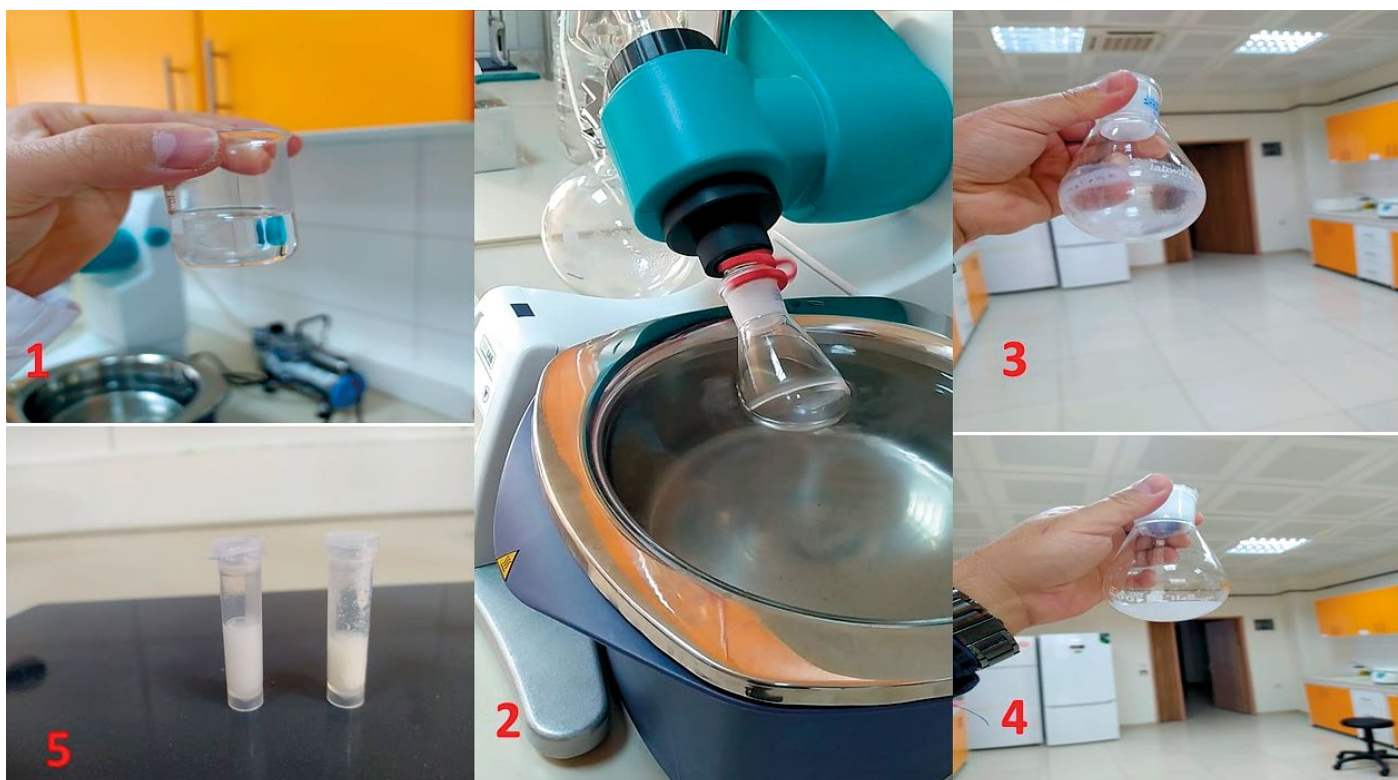
Fig. 1. Liposome preparation steps: 1 – dissolving substances, 2 – lipid film production in a rotary evaporator, 3 – lipid film obtained, 4 – lipid film retrieval, 5 – LVM
