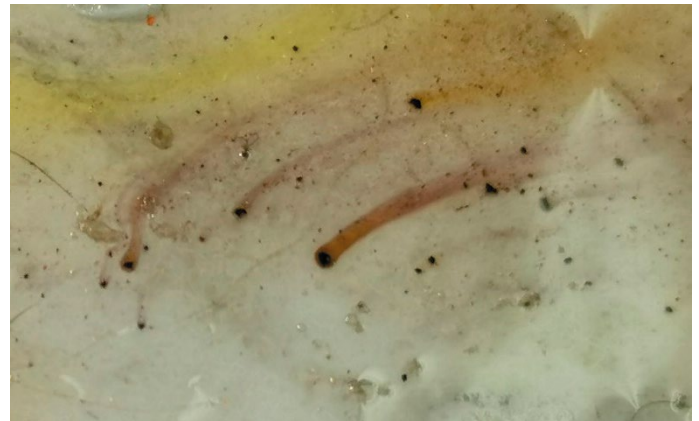
Fig. 1. Positive result for lead in a colour test for the presence of characteristic elements following a contact shot with .12 8.45 mm buckshot
