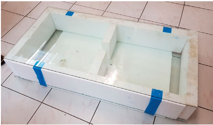
Fig. 1. Experimental chamber used in the behavioral avoidance assay. The terrarium measured 100 × 50 cm, was 15 cm high, and contained two 40 × 50 cm compartments connected by a 5 × 5 cm central corridor
